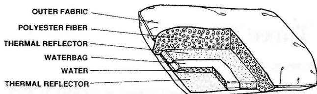
Fig 1. Diagram of cutaway view of cervical water-based pillow.<sup>a</sup>
